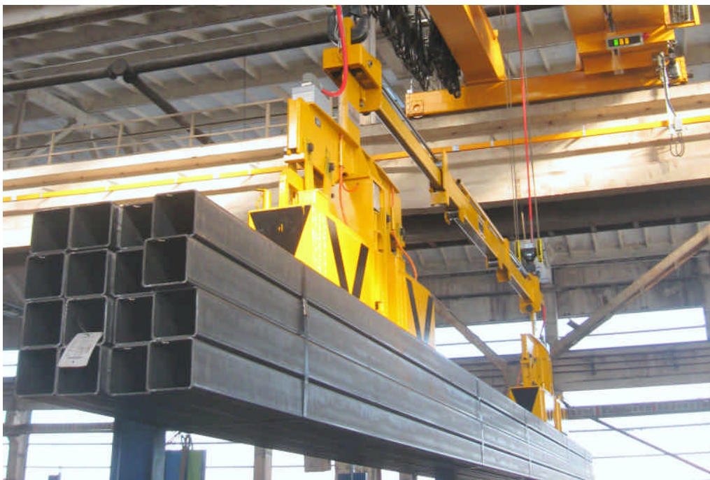
Figure 2: Plenty of power for safe and fast handling of hollow sections with the new TM magnet
