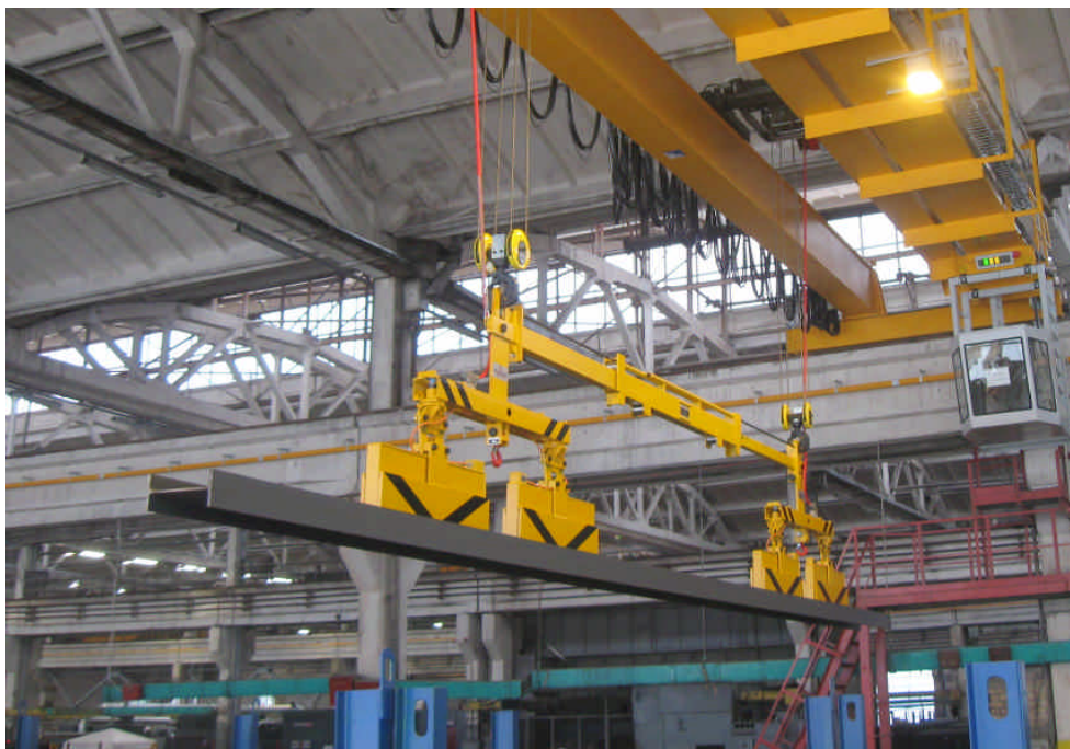
Figure 3: Passive telescope with narrow magnets for optimal beam handling
